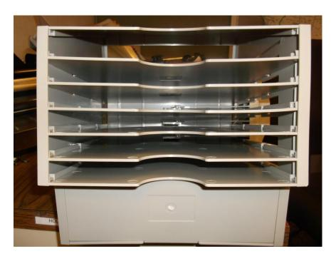
Moving the handle forward will move the arms forward and slide one piece of paper from each section forward so it may be removed from the unit.
