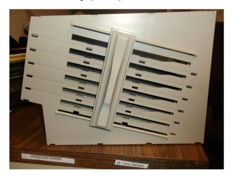
To reinstall the handle, line the handle up with the wide spots of the slots and push it back onto the machine.
