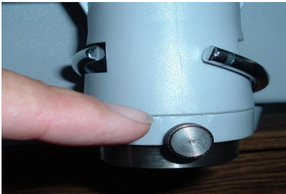
Step 1 loosen knob on output chute
