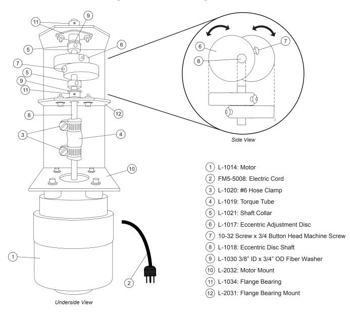
**Note:** When the screws are located opposite each other on the shaft, the minimum action is obtained. When the screws are located on the same side of the shaft, the maximum action is obtained. Normal action is obtained when the screws are 80° to 90° apart.
