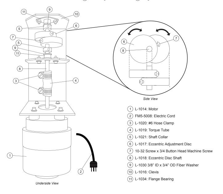
**Note:** When the screws are located opposite each other on the shaft, the minimum action is obtained. When the screws are located on the same side of the shaft, the maximum action is obtained. Normal action is obtained when the screws are 80° to 90° apart.
