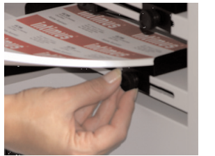
Fig. 6 Adjusting the paper guides
