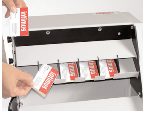
Fig. 13 Removing finished cards
