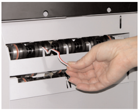
Fig. 15 Removing the jam
