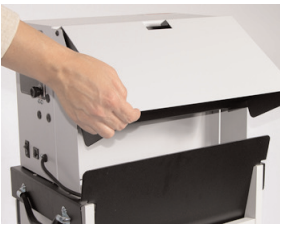
Fig. 14 Lifting the rear assembly
