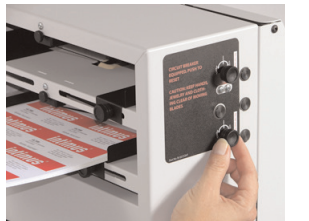
Fig. 7 Adjusting the retarder
