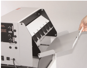
Fig. 4 Lowering the catch tray
