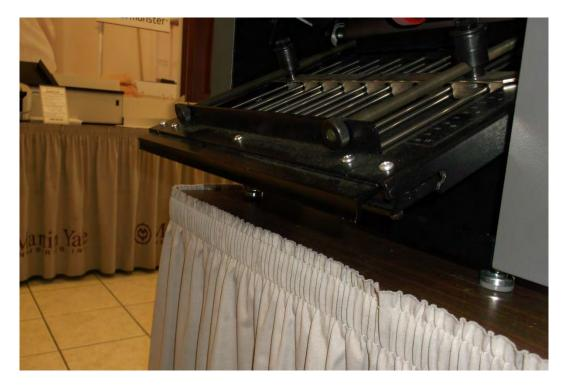
If you reverse both fold tables the paper goes through the machine without being folded. This is done when you are perforating or scoring the paper.
