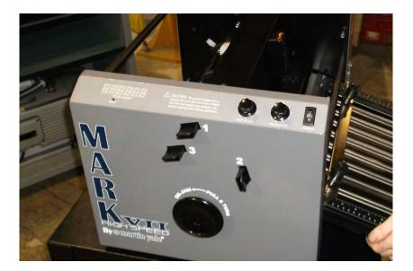
Using the paper you will be folding, cut 12 one inch x three inch strips. Insert the strips into the fold roller gap adjustment caliper as shown. You want one strip in slot 1, two strips in slot 2 and three strips in slot 3. If you are performing a double parallel fold insert four strips into slot 3.
