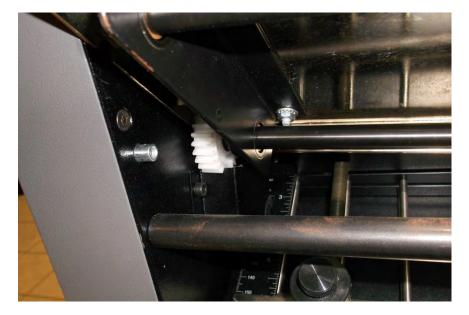
(gear not aligned in this picture)
