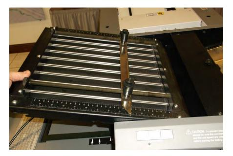
Install the first fold table by sitting the table on the locating pins and sliding it into place
