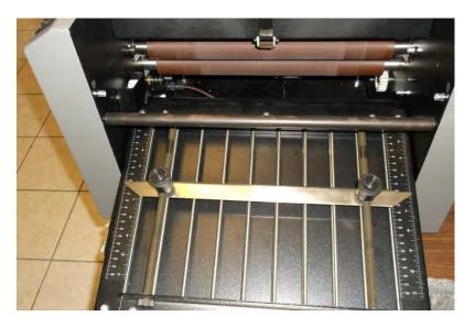
Install the second fold table under the feed tray
