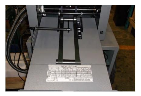
Set the stacking wheels according to the chart in the exit.
