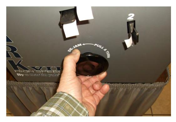
To assist in dejamming the machine, pull out on the dejam handle and turn in the direction of the arrow.
