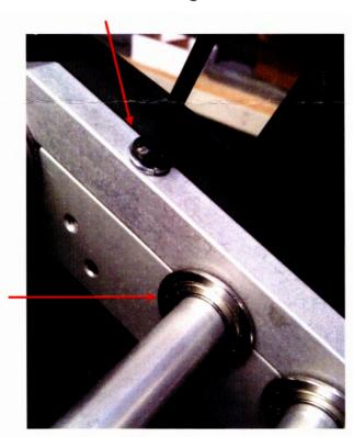
Before re-installing shafts, check to be sure the bearing retainer bolts on the end of shafts are tight.
